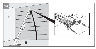
13 Insert anchor fittings (1). Lift the drive (2) at the front. Tightly fasten header fitting (3) at the front with two bolts (4) and U-washers (5).
