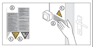
Please attach the warning signs (text + triangle sign) to a position where they are clearly visible, e.g. beside the pushbutton (warning triangle) and on the door wing (text + warning triangle).
