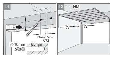
11 Make a mark 74 mm to the right and left of the center of the door (VM) and fasten at the same height on the header or ceiling (as per picture 9). Drill two holes (Ø 10 x 65 mm deep).
