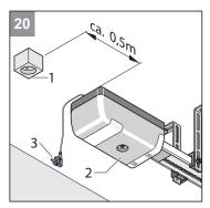
20 Install the socket (1) on the ceiling at a distance of approx. 0.5 m from the controller housing (2).
