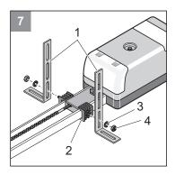
Mount the two steel brackets (1) with washers (4) and toothed lock washers (3) onto the ceiling holder (2).
