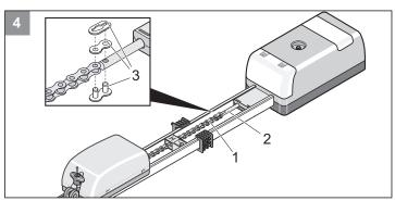
The chain (1) is connected to the chain attachment bolt of the controller housing (2) by means of the chain lock (3).
