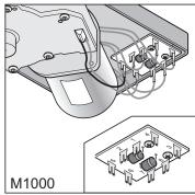
Terminal 1 Chain current draw Terminal 2 Rail current draw Terminals 3 + 4 Door OPEN Terminal 5 Motor cable Terminal 6 Motor cable
