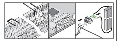
Green cable from Fraba system via photo eyes, only if DIP switch 2 ON. Terminal 6
