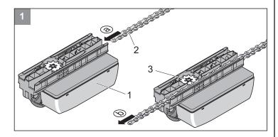
Insert the chain (2) from behind into the carriage (1). Ensure that the chain (2) lies correctly on the chain wheel (3).
