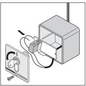
19 Install the key switch (1) in a suitable, easily accessible position in the garage. Minimum height above the ground: 1.6 m.
