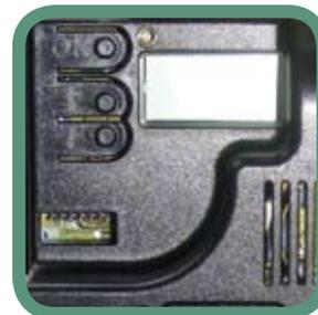
BUILT-IN PROGRAMMING DISPLAY AND RADIO RECEIVER
