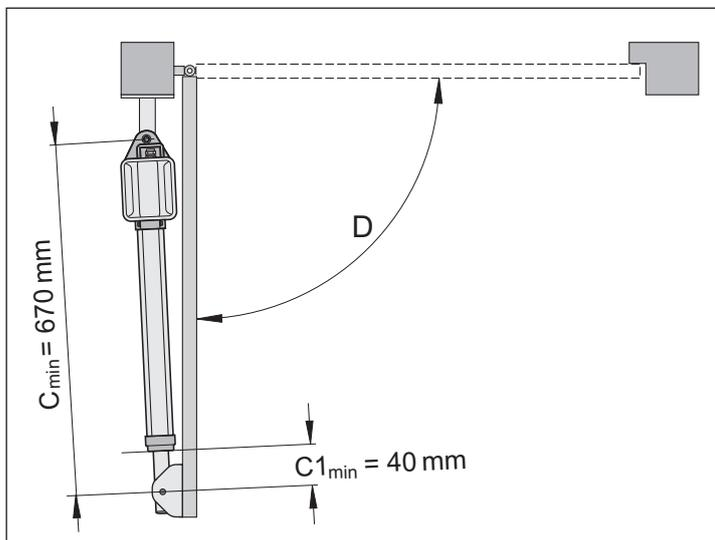
6. Manually move the gate to the "Gate OPEN" position. Note the maximum possible opening angle D from the A/B dimension table.
