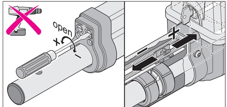
If necessary, readjust end position with a screwdriver.
