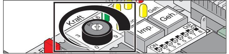
The force tolerance to the automatically learned force is set with the “P1” potentiometer.
