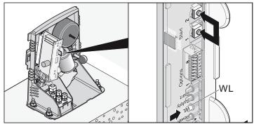
• Press and hold buttons (1 + 2) until the LED (warning lamp) is off
