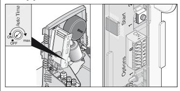
The GATE OPEN time can be adjusted at the potentiometer:
