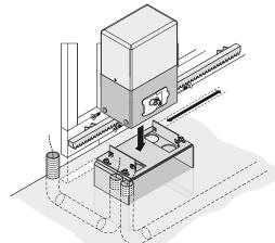
Mount the cover (2) and push it down. Turn key (1) 90° in anticlockwise direction and remove it.
