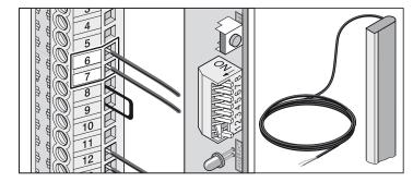
Terminal 6 + 7: Tested adapter for 8.2 kOhm resistor
