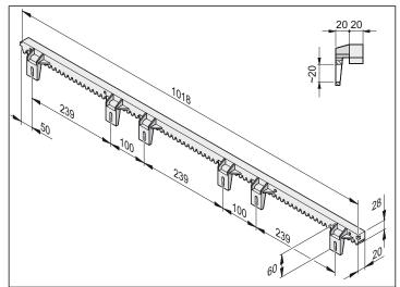
Mount the first rack at the opening edge of the gate. To mark the holes for the securing bolts, position the respective rack over the toothed wheel.
