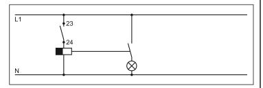
Example: Staircase lighting with automatic switching system
