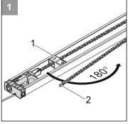
• Release the switch trigger (1) and move it in the direction of the arrow. Open the chain case (2).
