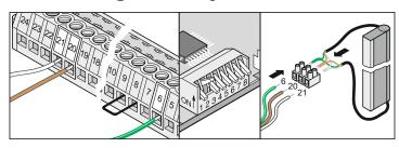
Terminal 6 Cable green from the Fraba system only if DIP switch 2 is ON
