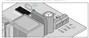
Connection strip for control cable that comes from the operator.
