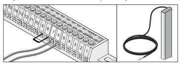
Terminals 6 + 7 Tested adapter for 8.2 kOhm resistor; DIP switch 2 set to OFF
