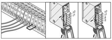
Terminals 8 + 9 Tested connection for potential-free contacts,
