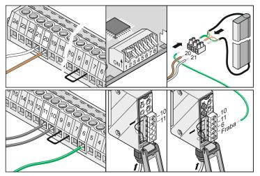
Terminal 6 Cable green from the Fraba system via photoelectric cell only if DIP switch 2 is ON
