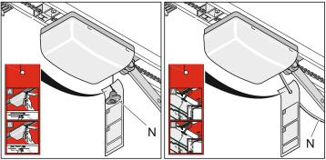
Attach the instruction label for the operation of the emergency release to the emergency release rope.
