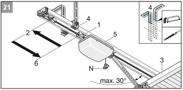
• Release rear switch-trigger buffer (1) and push right back to stop (2) Open door (3) by hand.
