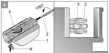
• Slide the trolley (1) onto the chain (2) with the chain case (4). The chain (2) engages in the chain wheel (3). If the chain wheel (3) does not turn, pull the emergency release (N) once. The chain wheel (3) is released.
