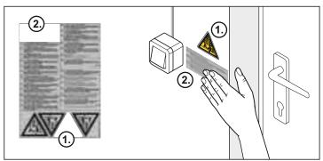
Attach the warning signs (text + triangle sign) at a position where they are clearly visible, e.g. beside the push button (warning triangle) and on the door leaf (text + warning triangle).
