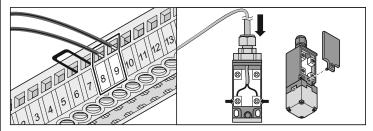
Terminals 8 + 9 Tested connection for potential-free contacts, only reacts if door is open
