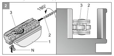
• Slide the trolley (1) onto the chain (2) with the chain case (4). The chain (2) engages in the chain wheel (3). If the chain wheel (3) does not turn, pull the emergency release (N) once. The chain wheel (3) is released.
