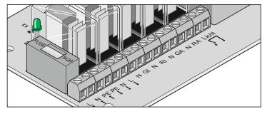
Connection strip for the signal lights (incl. mains supply) and potential-free relay contact (e.g. garage lighting).
