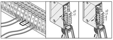
Terminals 6 + 7 tested connection for potential-free contacts,
