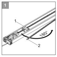
• Release the switch trigger (1) and move it in the direction of the arrow. Open the chain case (2).
