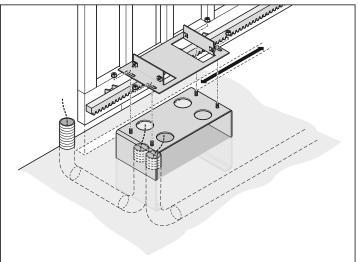
• Fix the anchoring plate to the console.
