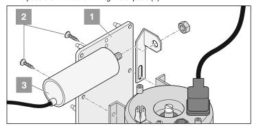
Push the capacitor (3) and its sheet metal holder between the motor and the control unit holder (1) and screw them together with 2 screws (2).
