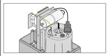
The slipping clutch slips when an obstacle is encountered (drive stops). After the preset running period, the drive switches off.
