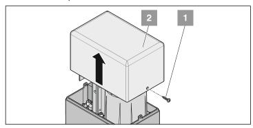
· Loosen screws (1). Remove lid (2).
