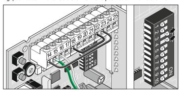
Radio channel 1 always has the same function as push-button 1, terminal 20 + 21.
