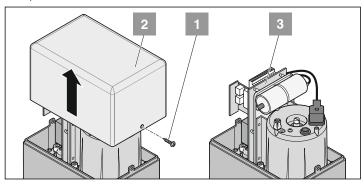
• Loosen screws (1). Remove lid (2).
