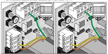
Please detach the cable for the end switch from the green terminal and connect it to the new control unit. For connections see below.
