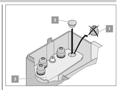
• Remove the screw cable connection (1) and block the hole with a plug (2). Screw cable connection (1) has no counternut, removal is possible without removing metal plate (3).
