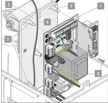
Insert T100 control unit (1) and screw together with the control unit holder (3) using 2 screws (2). Lead the cable (4) for the magent end switch upwards between the T100 control unit and the control unit holder.
